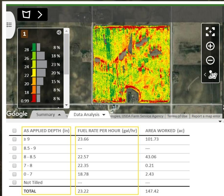
Deeper tillage depth resulted in higher fuel rates per hour
